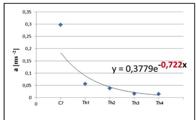
Fig. 5. Dependence of the acceleration size detected at the vertebrae of the spinal segments C<sub>7</sub>–Th<sub>4</sub> – before the loading. The coefficient  $b = 0.772$ , see the 2nd row in Table 2.
