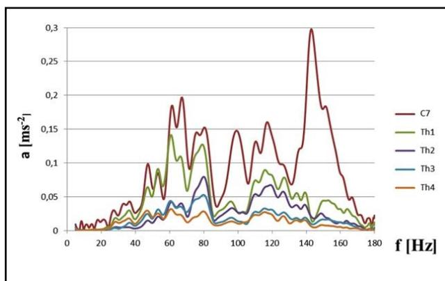
Fig. 4. AS frequency response of the section C<sub>7</sub>–Th<sub>4</sub> monitored – before loading
