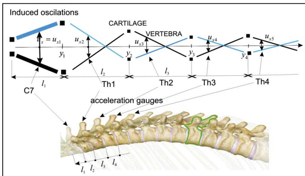
**Fig. 3.** Geometric scheme of the oscillating AS components and their parameterization.  $u_x$  – deflection of the oscillating motion segment [m];  $y_i$  – vertebrae coordinates [m];  $l_{1,2,3}$  – vertebral heights [m]; C<sub>7</sub>, Th<sub>1</sub> – vertebra
