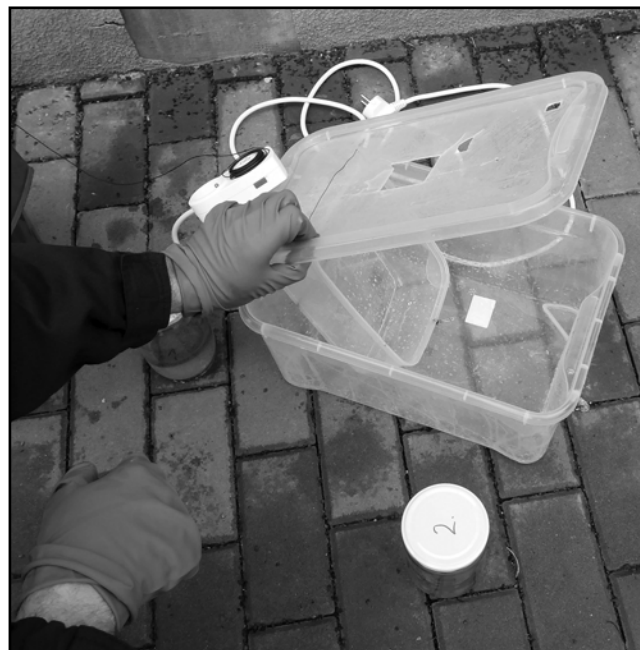
Fig. 1. Double-container apparatus used for generation of carbon monoxide.
