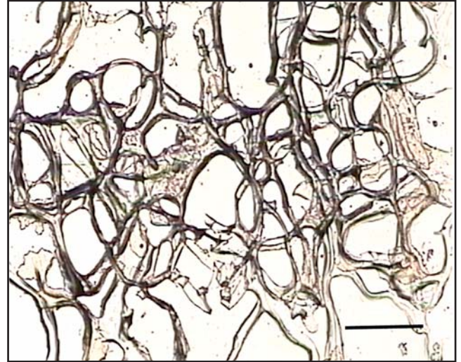
Figure 1. A thin slice of freeze-dried chitosan scaffold. Chitosan formed a sponge-like 3-dimensional structure that was highly porous. Pores ranged from 50–350 \mu\text{m} wide. Scale bar, 200 \mu\text{m} .
