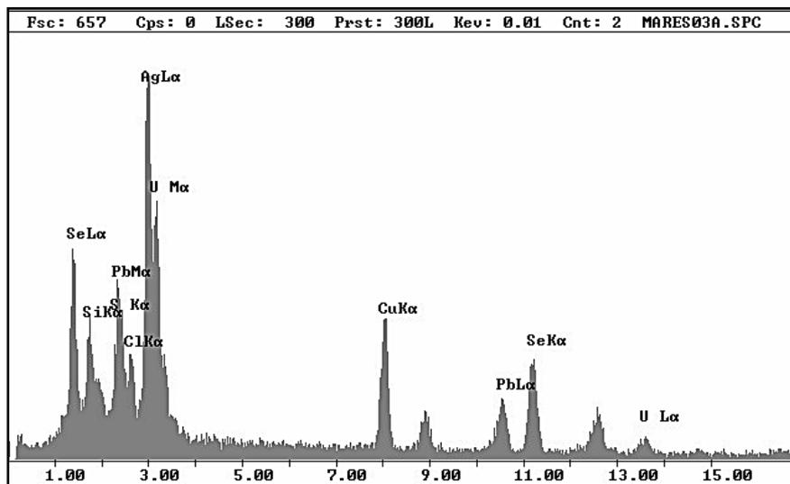
**Figure 5.** Characteristic X-ray spectrum recorded from typical electro-dense particle in the ultra-thin section (see particle marked with asterisk in Fig. 2) with the content of Ag, S, Se. The other elements recorded in spectrum originate from sample preparation process (Cl, U, Pb, Si) or from support grid (Cu). Background spectrum recorded near the analysed particle. x – axis: energy in keV; y – axis: counts
