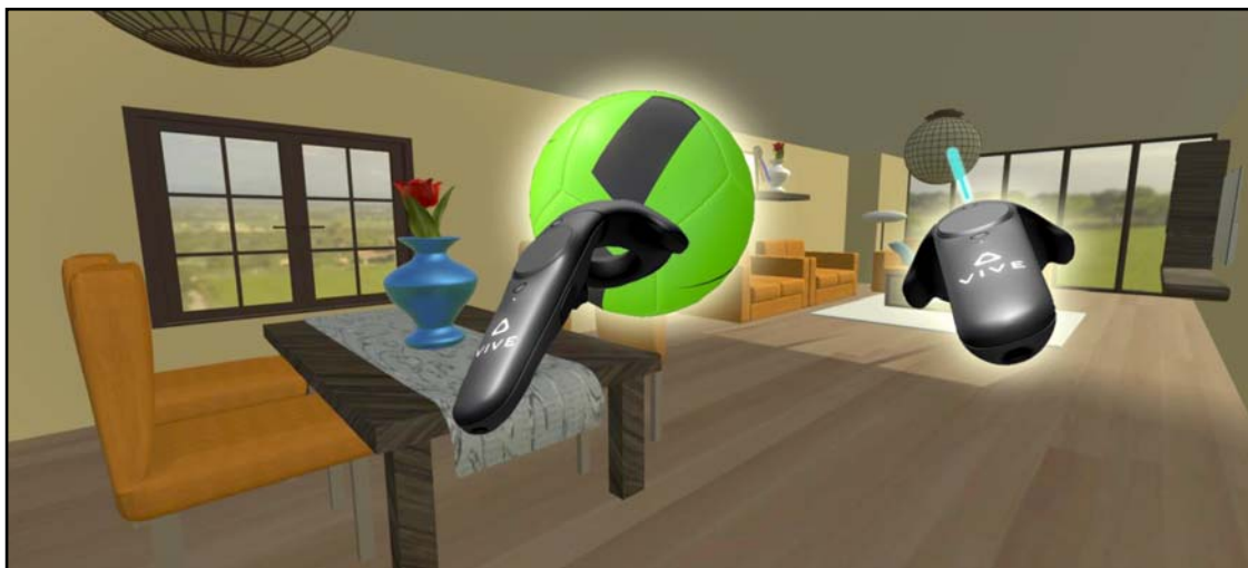
Fig. 1. Virtual environment of one of the scenarios. Ball is assigned to the left controller. The path of the ball is calculated based on the speed of the controller as it moves by the user. The right controller displays a pointer to an object in the scene that can be interacted with. (Source: own research)
