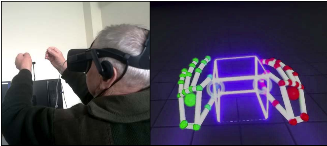
Fig. 2. Rehabilitation of fine motor skills of the upper limbs. The user's physical movement is shown on the left. On the right is a virtual scene with a virtual skeleton obtained using sensors rigged to the 3D hand model when using Blocks application for Leap Motion sensor. (Source: own research)
