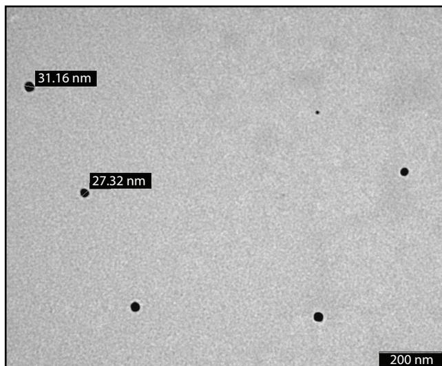
**Fig. 1.** Electron-microscopic image of silver nanoparticles stabilized with 0.01% solution of maltose and gelatine.
