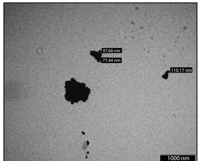
**Fig. 2.** Electron-microscopic image of silver nanoparticles stabilized with polyvinylpyrrolidone.
