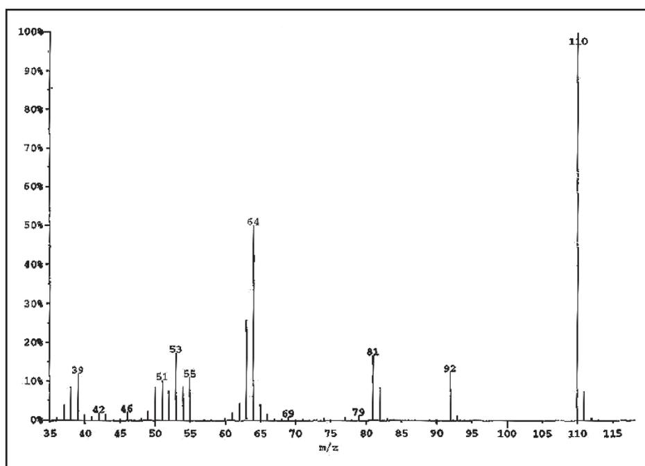
**Fig. 2.** Mass spectrum of a phenol metabolite formed by extracellular phenol hydroxylase of the medium used for cultivation of *C. testosteroni*.
