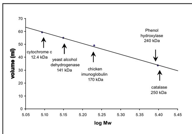
**Fig. 5.** Molecular mass determination of extracellular NADPH-dependent phenol hydroxylase of *C. testosteroni* by gel permeation chromatography on Sephacryl S-300. Experimental conditions are described in Material and methods.
