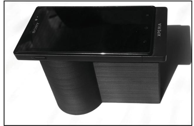
**Fig. 1.** Instrumental arrangement of the smartphone and our designed and made holder for taking snapshots of the samples.
